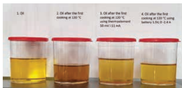
Figure 4 Oil before frying (1), after frying at 120°C (2), after frying at 120°C using a thermocouple (3) and after frying at 120°C using a battery (4), [6]
